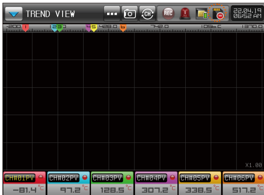
[Fig. 6-3] The screen not available for saving in case of no insertion of the card
