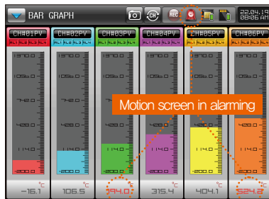
[Fig. 14-12] Operation screen for bar alarm creation
