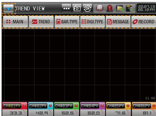
[Fig. 4-2] Screen in case of non saving the graph (Display of sub menu bar)
