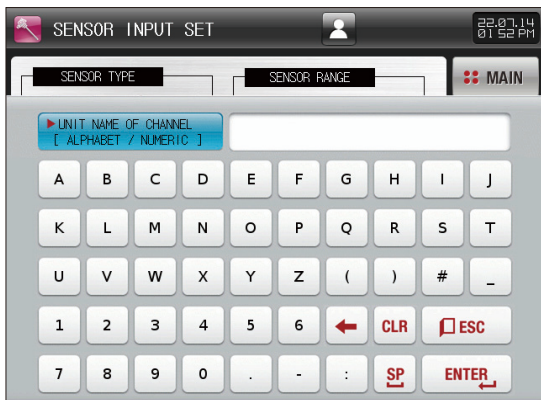
[Fig. 13-12] Screen for name setting by setting the display unit with editing
