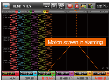
[Fig. 14-10] Operation screen for vertical axis alarm creation
